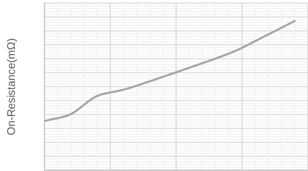
Figure 11. Channel-4 FET On-Resistance VS Temperature
